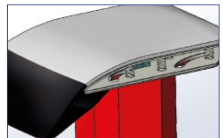
Close-up of springs giving a fast, dynamic response
