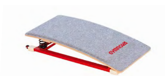
Ref. 2190 Training springboard - 21 cm Supplied with 2 firm cylindrical springs and a board covered with a 2 cm thick carpet mat. Height: 21 cm, weight: 24 kg.
