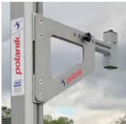
weatherproof anodized aluminium profile, aluminium crossbar support with horizontal adjustment range 0-15 cm, support runner based on eight ball bearings guarantees smooth work of crossbar raising mechanism
