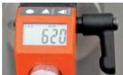
implementation of electronic height indicator begins a new era of constructing PV standards, original Polanik solution has removed a traditional measuring tape, hermetic indicator casing with stainless steel hub installed on crank, resistant to high temperature and humidity, resistant to UV radiation and chemical agents, equipped with brake, battery life min. 5 years
