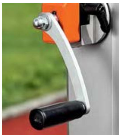
weatherproof anodized aluminium profile, aluminium crossbar support with horizontal adjustment range 0-15 cm, support runner based on eight ball bearings guarantees smooth work of crossbar raising mechanism
